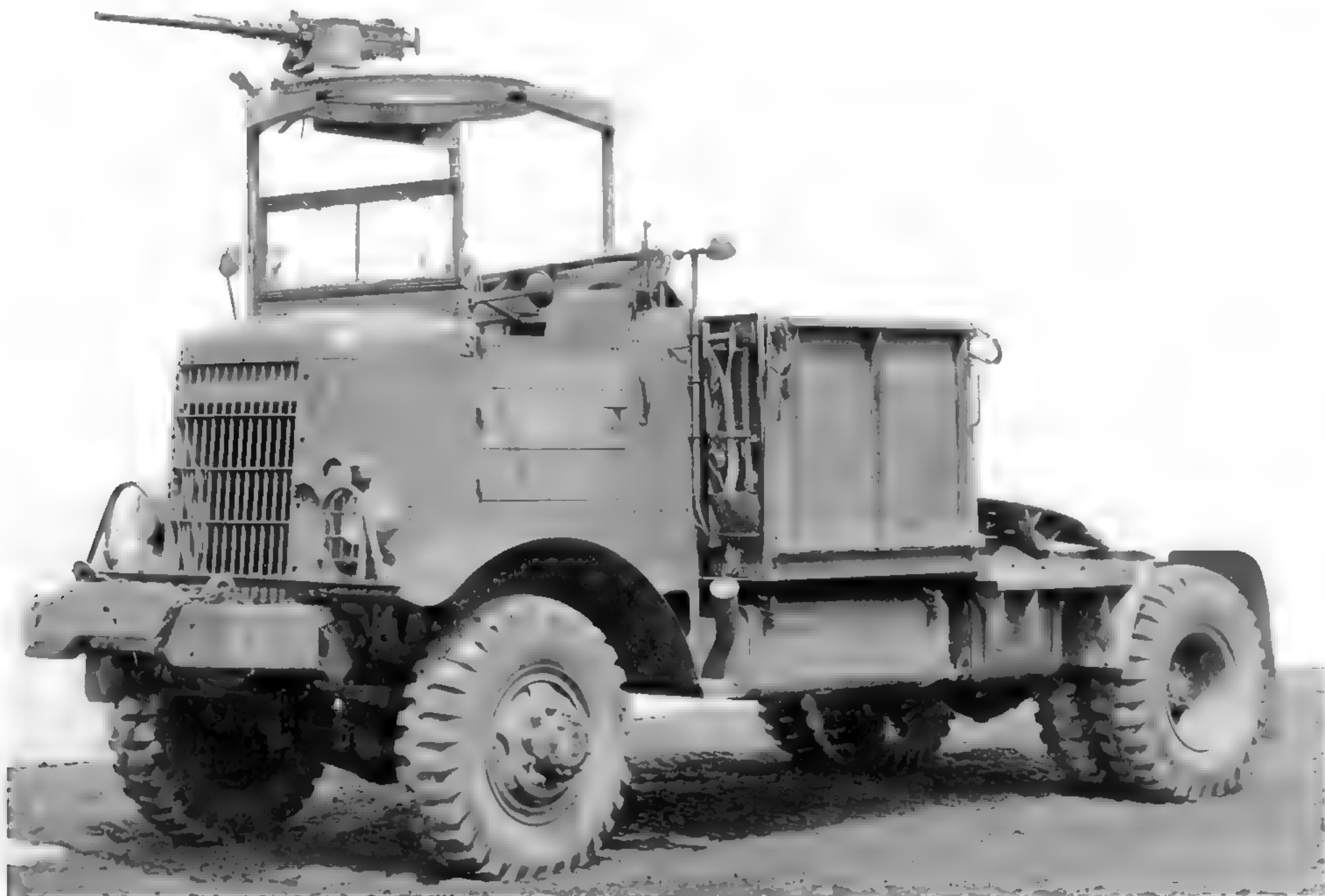
The U-8144-T could be fitted with an antiaircraft ring mount. (U.S. Army photo)
